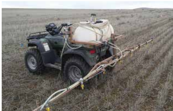
Equipment used for sulfentrazone (Spartan® Charge) application to field research plots.
