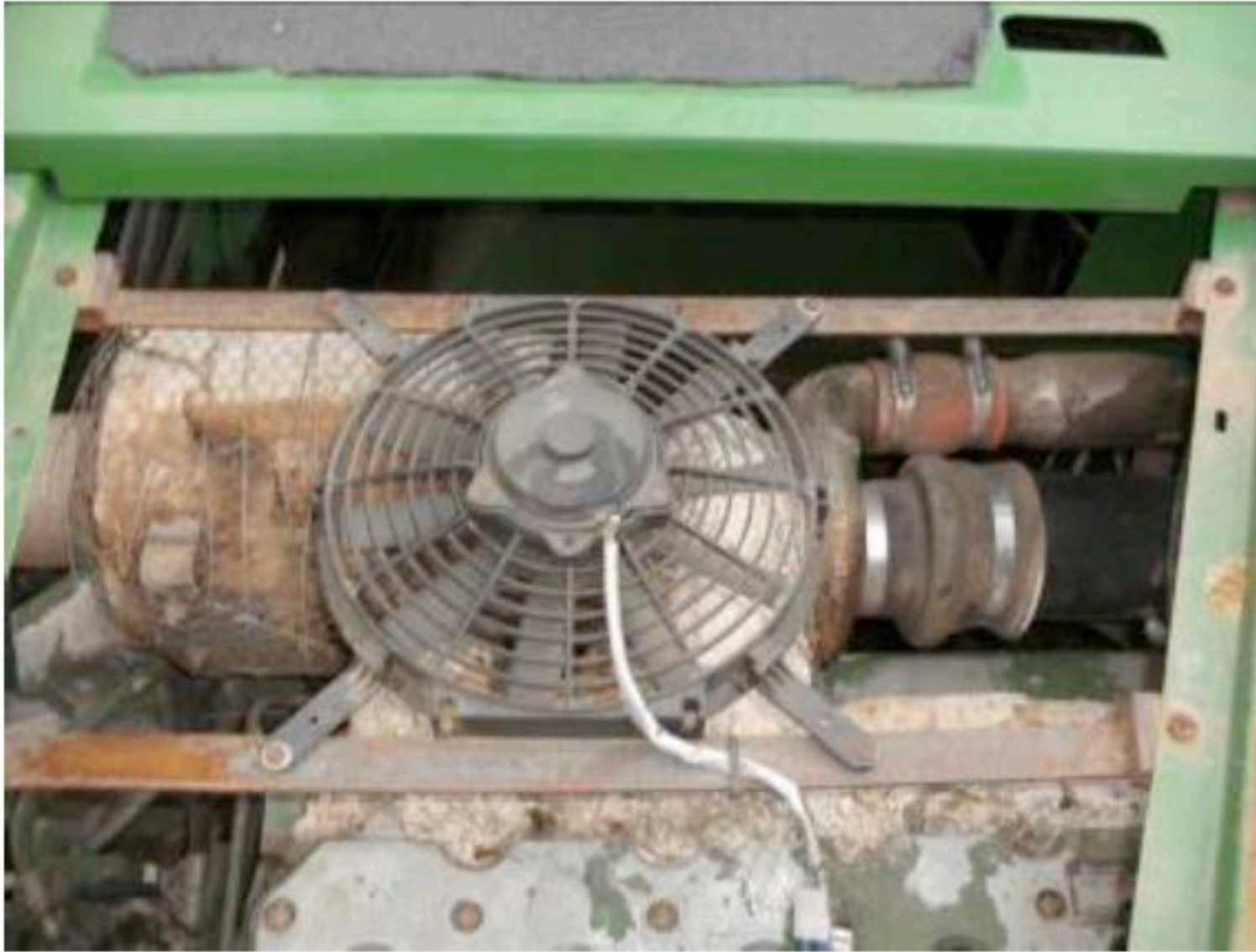
Fig 9. Engine bay modifications. This is a farmer-installed extra fan (ex-Auto) and insulation wrapping around the exhaust system on an STS by Custom Contractor Harry Roper in Goondiwindi. The non-standard shield wrapped around the exhaust system has not caused any turbo problems so far but it is not a Company authorized fitment.
